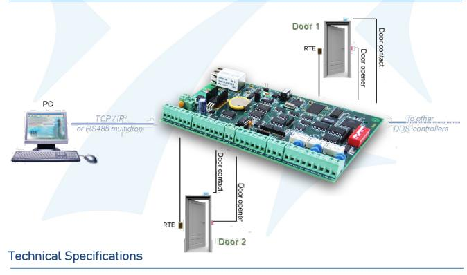
Operating temperature: 0° C to +55° C Storage temperature: -10° to +65° C Operational humidity: 10 to 95% RH Working voltage: 12 VDC +/- 20% 350mA with TCP Alarm input max voltage:+/- 30V
